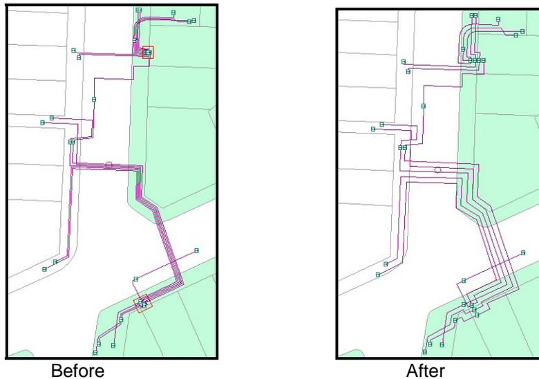
■ The Geo-Linear Dispatch layout algorithm has been enhanced by moving leaves with one link. To get the clearest diagrams, the layout is enhanced to include the leaves having one link in the repositioning process. This function is useful to manage secondary networks in the field of water, gas and electrical distribution: (*This enhancement was originally introduced in 9.2 Service Pack 3*):
